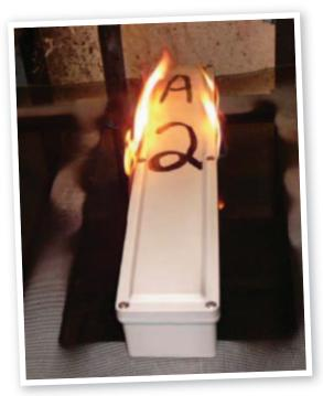
Stahlin Non-Metallic Enclosure CF Series during the UL 2043 testing
