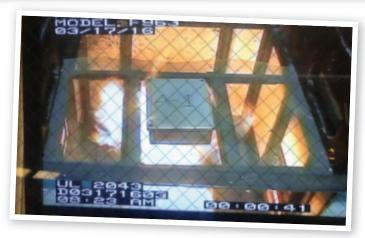
The Stahlin F Series Non-Metallic Enclosure during testing for UL 2043
